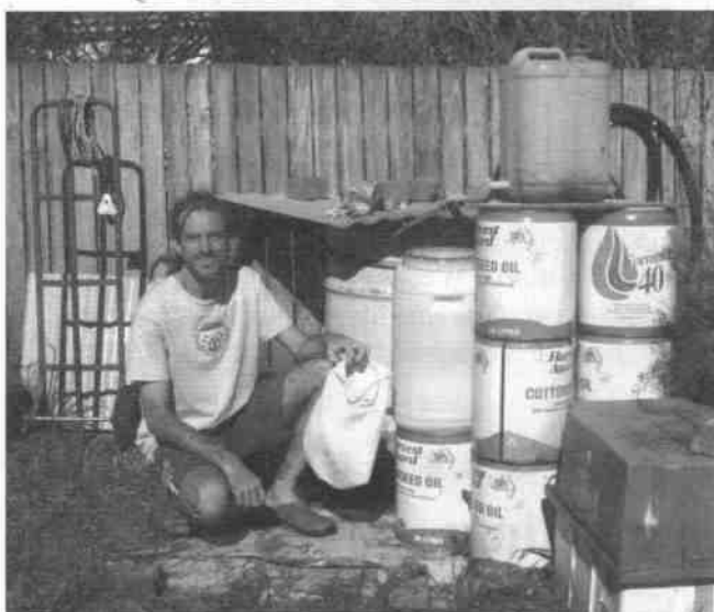
Benny in front of used vegetable oil drums and filtering apparatus, holding the 5 micron filter sock
